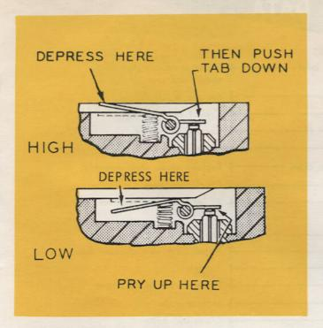
be bent, extruded from being forced into the casting seat or possibly broken off in the casting. If either mixture screw is damaged, be sure to inspect the condition of the casting. If the adjustment seats are damaged, a new body casting is required.
