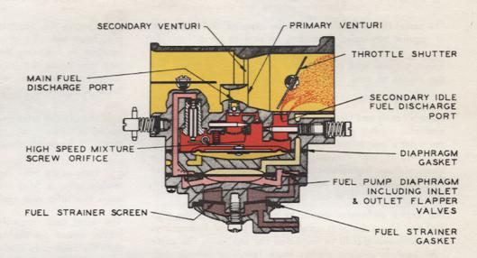
existing within metering diaphragm fuel chamber, fuel is drawn up through high speed mixture screw orifice and out main fuel discharge port.
